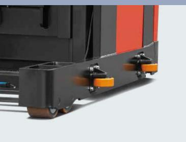
Rail guidance rollers (Opt.) can be fitted to the truck for VNA working
